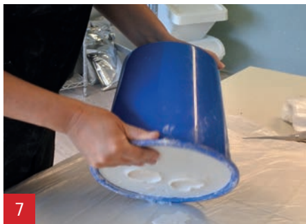
7 Carefully turn the bucket over so the cured alginate slides out of the bucket with the cured A1.
