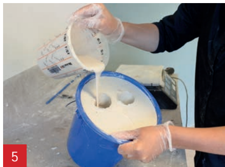
5 Slowly pour some of the A1 along the edge into the opening(s). Let the A1 flow through the shape in all directions to reduce air entrapment. Turn and tap on the bucket so the A1 fills the void properly and any air bubbles rise. Pour in the remaining A1. Again, tap on the bucket and fill to where necessary.
