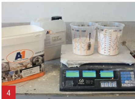
4 Weigh 1 part A1 Liquid and 2 parts A1 Powder and mix. The A1 is ready as soon as you run out of lumps or air bubbles.
